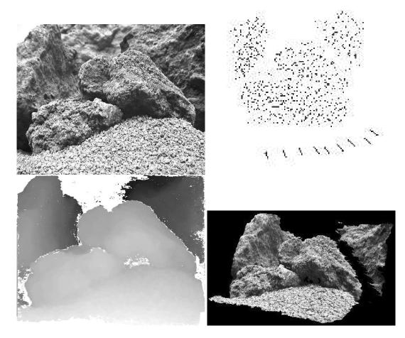
Figure 9.27: Different steps of the 3D reconstruction of a rock from images.
