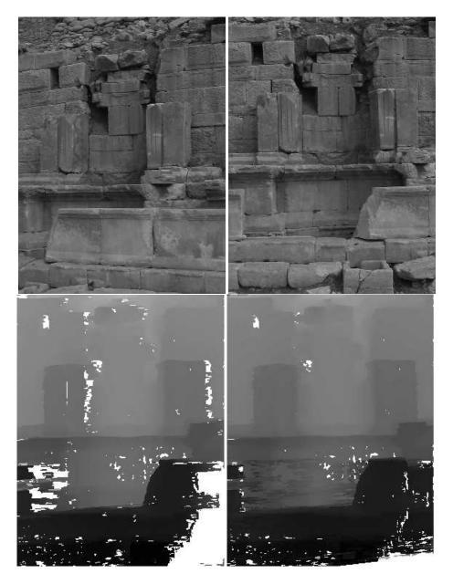
Figure 7.19: First and last image of fountain sequence (left). Depth maps from the 2-view and the 5-view estimator (from left to right) showing the very dense depth maps (right).
