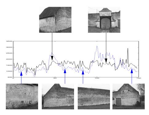
Figure 5.10: Some images of the *farmhouse* sequence together with GRIC(**PPP**) (solid/black line) and GRIC(**HH**) (dashed/blue line).
