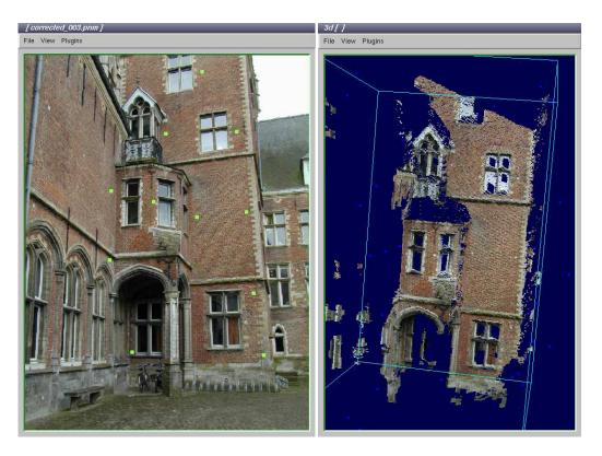
Figure 9.23: On the left one of the input images can be seen with the measured reference points superimposed. On the right the cloud of reconstructed points is shown.
