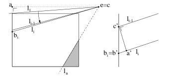
Figure 7.6: Determining the minimum distance between two consecutive epipolar lines. On the left a whole image is shown, on the right a magnification of the area around point  $b_i$  is given. To avoid pixel loss the distance |a'c'| should be at least one pixel. This minimal distance is easily obtained by using the congruence of the triangles abc and a'b'c'. The new point b is easily obtained from the previous by moving  $\frac{|bc|}{|ac|}$  pixels (down in this case).
