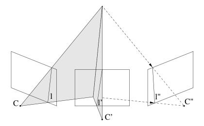
Figure 3.8: Relation between the image of a line in three images. While in the two view case no constraints are available for lines, in the three view case it is also possible to predict the position of a line in a third image from its projection in the other two. This transfer is also described by the trifocal tensor.
