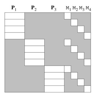
Figure A.1: Sparse structure of Jacobian for bundle adjustment.
