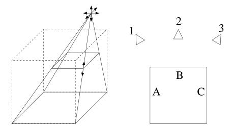
Figure 5.5: Left: Illustration of the four-parameter ambiguity between two projective reconstructions sharing a common plane. If the base of the cube is shared, a projective transformation can still affect the height of the cube and the position of the third vanishing point. Right: A fundamental problem for many (manmade) scenes is that it is not possible to see A,B and C at the same time and therefore when moving from position 1 to position 3 the planar ambiguity problem will be encountered.
