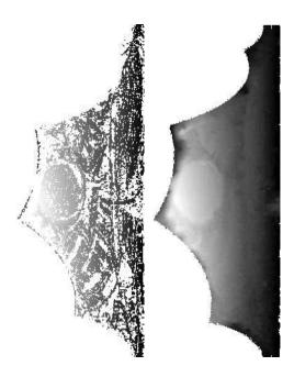
Figure 7.12: Raw and interpolated disparity estimates for the far image of the desk image pair.
