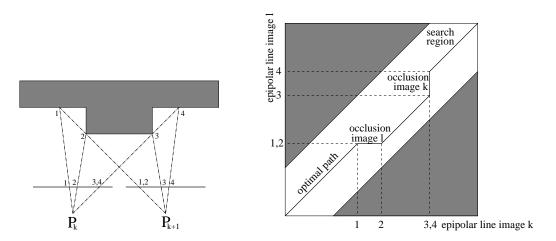
Figure 7.14: Object profile triangulation from ordered neighboring correspondences (left). Rectification and correspondence between viewpoints k and l (right).
