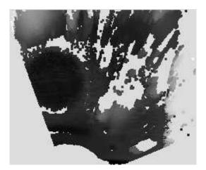
Figure 9.26: Digital Elevation Map of the ESTEC planetary testbed. A significant amount of cells is not filled in because they are located in occluded areas.
