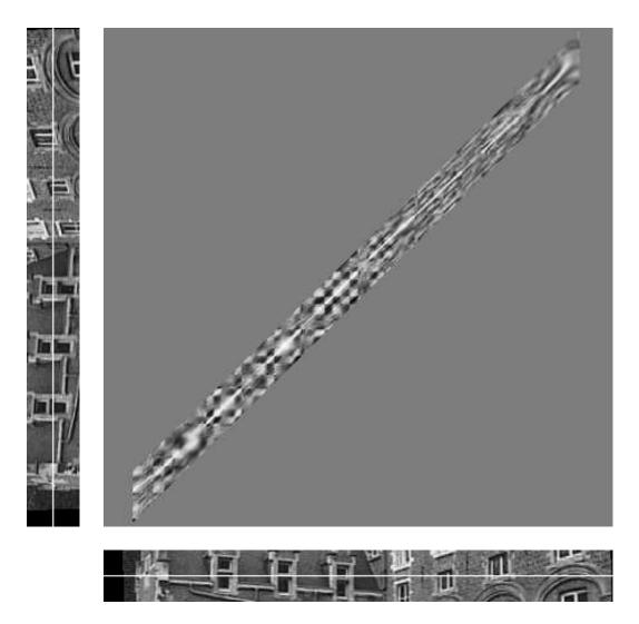
Figure 7.16: Cross-correlation for two corresponding epipolar lines (light means high cross-correlation). A dynamic programming approach is used to estimate the optimal path.
