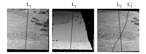
Figure 9.24: Digital Elevation Map generation in detail. The figure contains the left rectified image (left), the corresponding disparity map (middle) and the right rectified image (right). The 3D line L corresponding to a point of the DEM projects to  $L_1$  resp.  $L_2$ . Through the disparity map the *shadow* of  $L_1$  on the right image can also be computed. The intersection point of  $L_2$  and  $L_1$  corresponds to the point where L intersects the surface.
