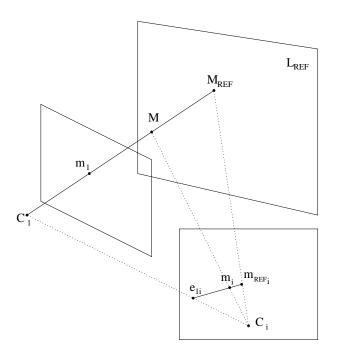
Figure 3.4: A point M can be parameterized as  $C_1 + \lambda M_{REF}$ . Its projection in another image can then be obtained by transferring  $m_1$  according to  $\Pi_{REF}$  (i.e. with  $\mathbf{H}_{1i}^{REF}$ ) to image *i* and applying the same linear combination with the projection  $\mathbf{e}_{1i}$  of  $C_1$  (i.e.  $m_i \sim \mathbf{e}_{1i} + \lambda \mathbf{H}_{1i}^{REF} \mathbf{m}_1$ ).
