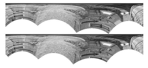
Figure 9.7: Rectified image pair (corresponding pixels are vertically aligned).
