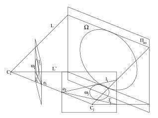
Figure 6.2: The Kruppa equations impose that the image of the absolute conic satisfies the epipolar constraint. In both images the epipolar lines corresponding to the two planes through  $C_i$  and  $C_j$  tangent to  $\Omega$ must be tangent to the images  $\omega_i$  and  $\omega_j$ .
