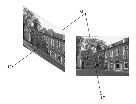
Figure 1.3: Reconstruction of three-dimensional point through triangulation.
