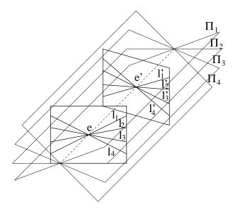
Figure 7.2: Epipolar geometry with the epipoles in the images. Note that the matching ambiguity is reduced to half epipolar lines.
