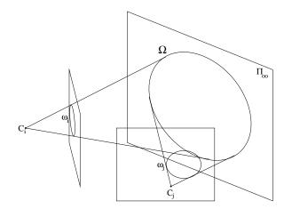
Figure 6.1: The absolute conic (located in the plane at infinity) and its projection in the images
