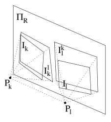
Figure 7.1: Planar rectification:  $(\mathbf{I}_k^l, \mathbf{I}_l^k)$  are the rectified images for the pair  $(\mathbf{I}_k, \mathbf{I}_l)$  (the plane  $\Pi_R$  should be parallel to the baseline  $(\mathbf{P}_k, \mathbf{P}_l)$ ).
