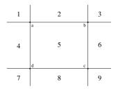
Figure 7.4: the extreme epipolar lines can easily be determined depending on the location of the epipole in one of the 9 regions. The image corners are given by a, b, c, d.
