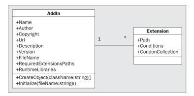
The attributes shown in the diagram above are populated from the add-in XML file that we saw in the *Add-in Definition* section. The extensions contained in the add-in XML are stored in a separate class called Extension that contains all extension paths and contents defined by this add-in. An extension path is just a shortcut for putting codons in the appropriate path.
