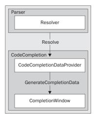
This diagram shows why the Resolver can be considered as being outside the scope of the Parser. The Resolver is elementary for code completion; it provides the base for actually using the parse information for the file in the edit buffer.
