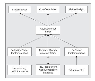
We can see that we have three consumers of data, as well as three providers of data; each with its own specific parser. This is necessary, as we need to know quite a lot for successful parsing of the code. Not all elements in our code are contained in the specific file that we edit; we use .NET reflection to handle references to assemblies and the .NET Famework.
