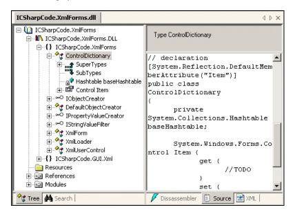
Here, we can see the source code for the same DLL file. If the source code isn't available then the pane will simply display Source view not available. Since we do not have a decompiler available, we can only see the skeleton of the code. Clicking the XML tab will display the following:
