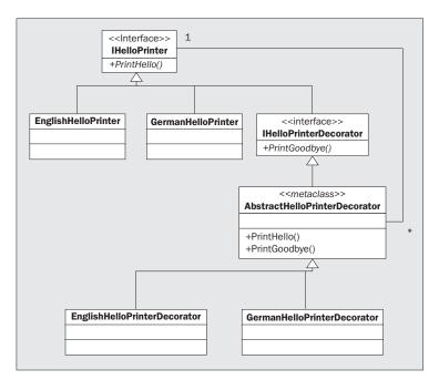
In this diagram, we can see that the real HelloPrinter classes can inherit from another class without problems. Other decorators can be added to it without problems. The HelloPrinters can change their decorator at run time and extend their functionality dynamically.
