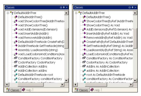
With the C# ambience shown on the left the methods and fields are printed in C# style (type first; look at the method parameters and return values). The VB.NET ambience shown on the right prints the names in VB.NET style (name As Type).
