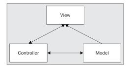
As we can see from the diagram, the controller is between the view and the model and it communicates with both of them. The view needs to display the data. Therefore, it needs to read the model. It does not need to make changes to the model so this communication is one-way.
