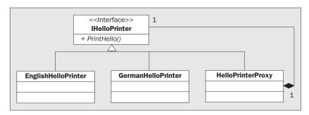
As we can see from the diagram, the proxy class is just an implementation of the interface that the actual big class implements. The classes that use HelloPrinters don't know the difference between the proxy implementation and the real ones.
