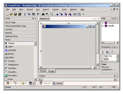
The Tool Scout, selected by the Tools tab, allows us to click and drag Windows Form Controls onto the previously created blank form. After we have some Controls on the form, we will need to edit their properties.
