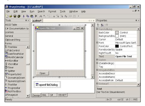
This Designer area contains four components: the form, textbox, and button, which are the visible ones, and the openFileDialog (invisible). We need a format that can describe all the properties of the components, and can recognize the location of the components. For example, the button and textbox are child controls of the form.
