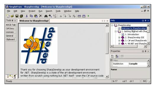
The Properties pad's default location is at the right-hand side below the Help pad (see previous screenshot). The properties pad contains a list of the properties of the currently opened item. For example, if a file is currently visible in the main window, the pad lists the respective properties of the file or if a Windows Form Control is selected you can edit the control's properties:
