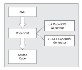
The XML is transformed into CodeDOM data structures by using the code generators (provided by the framework).
