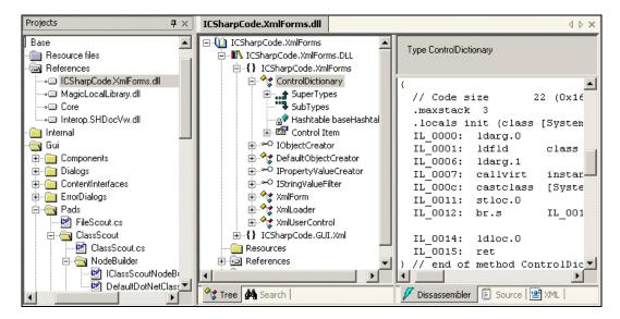
In the screenshot, the Assembly Scout was started by double-clicking a reference in the Project Scout. It consists of two panels. The first one is a tree view representing classes and members, similar to the Class Scout, grouped with a Search tab in the left hand pane. The right-hand pane contains information about the tree node that is highlighted in the left-hand pane. This pane offers three tabs for displaying information.
