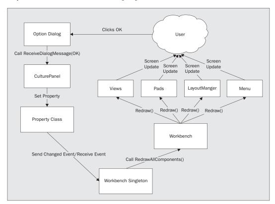
This simplified flowchart shows us the sequence from the user's click to the redrawn GUI. After the user confirms their selection by pressing the OK button, the AcceptEvent method (located in the TreeViewOptions.cs file under src\SharpDevelop\Base\Gui\Dialogs) triggers a DialogResult.OK message. The message is received by the ReceiveDialogMessage method located in the src\SharpDevelop\Base\Gui\Dialogs\OptionPanels\IDEOptions\SelectCulturePanel.cs file:
