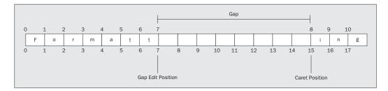
The numbers above the boxes are the user co-ordinates, as they represent the user's view of the edit buffer, and the ones below are the gap co-ordinates used internally in handling the buffer. Both co-ordinate systems refer to the locations between the characters in the buffer. The user and the caret see the user co-ordinates only, which are used in our implementation independent of the internal state of the gap.
