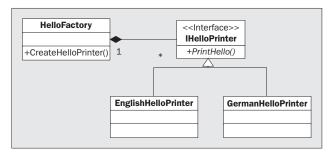
This is the UML diagram for our example. With this pattern, we can easily add new concrete HelloPrinter classes to our HelloFactory that can be created without letting the users of the factory know that other implementations are added. The classes that use HelloPrinter classes only need to know the factory class.
