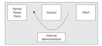
The general flow of information, in a parser, goes from the input to the partial parse trees, as output. It affects, and is affected by, the control and internal administration of the automaton. Usually, all the parts of a parser are affected by each step that is performed.
