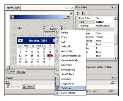
The Control's properties are located on the left on the default setting. Of course, we can rearrange the panels as SharpDevelop supports Window docking. The property panel allows us to edit the Controls in a very intuitive way.
