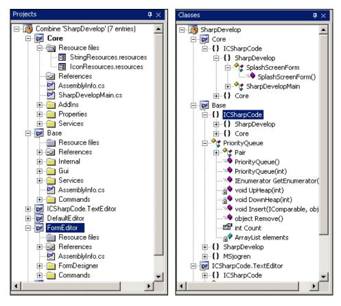
The Project Scout allows easy navigation and assignment of various settings of its items by right-clicking on the entry – a file, project, or combine.
