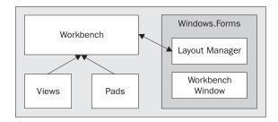
The abstract GUI layer is simple. We have a Workbench that contains views and pads, similar to a container. The views are windows having editable content, like text. Pads, on the other hand, are tool windows, like the Project Scout.
