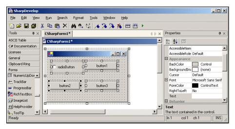
Note that the button2 component is surrounded by small black squares, whereas for the other selected components they are white. This indicates that button2 is a special component, or the primary selection. The Selection service must have a way to handle the primary selection, as well as the other selected components.
