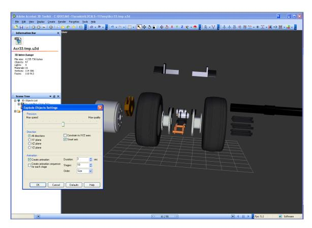
Use the Explode Objects Settings dialog box to tailor factors such as speed, direction, duration, and number of stages in a typical exploding-parts animation.
