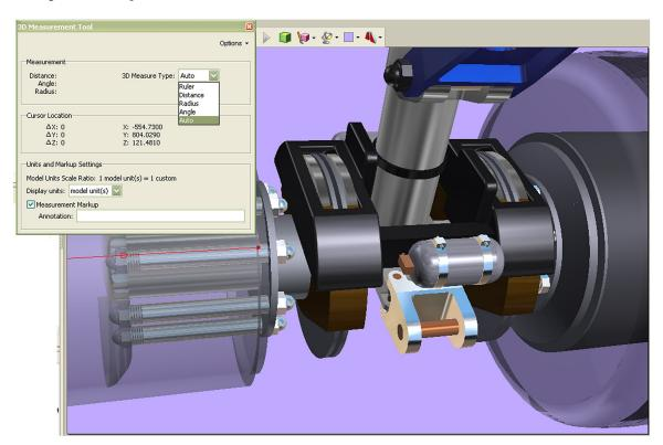
The Distance tool, visible as the red line in this image, allows you to take precise measurements in any model. Adjust units and track precise cursor location in the 3D Measurement Tool dialog box, and set the 3D measurement type to assist in measuring radius, angle, distance, and more, simply by dragging across the 3D model.
