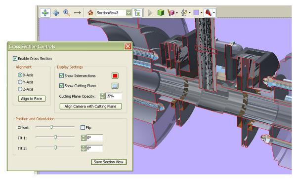
Create detailed cross-section views in Acrobat 3D to interrogate 3D models as deeply and in as much detail as you need, complete with fine controls for the cutting plane, alignment, and orientation. Save as many section views as you choose, with one click each of the Save Section View button.
