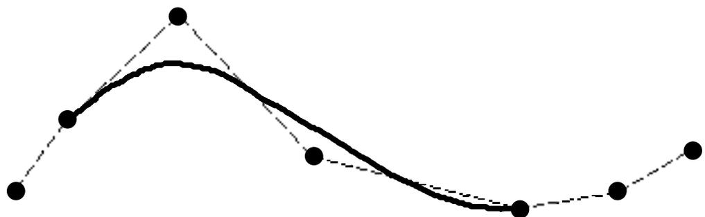
There is no spline data generated for the first and last two control points
