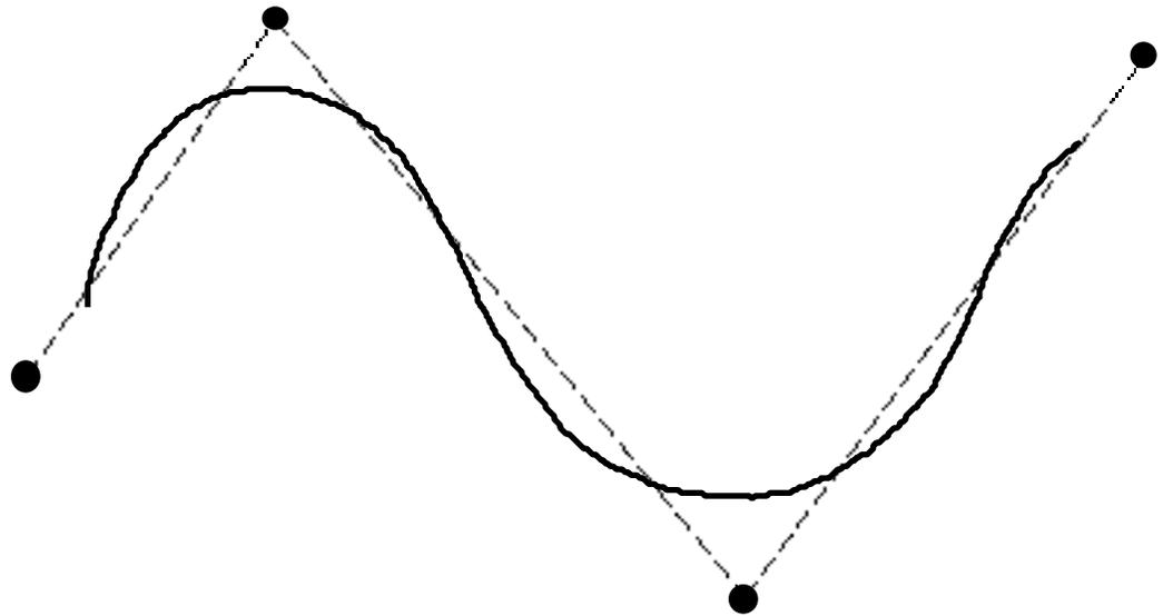
A b-spline does not pass through it's control points
