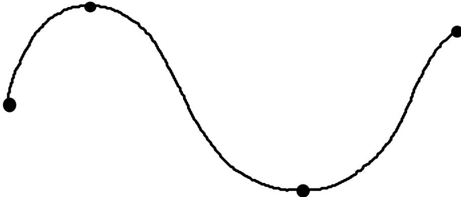
A cubic spline passes through it's control points
