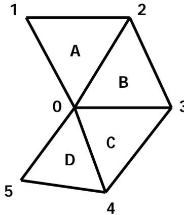
Here, triangle A is drawn by passing vertices 0, 1, and 2 to the 3D hardware. Next, to draw triangle B, only vertex 3 needs to be passed since the hardware will use vertices 0 and 2 from the previous triangle.
