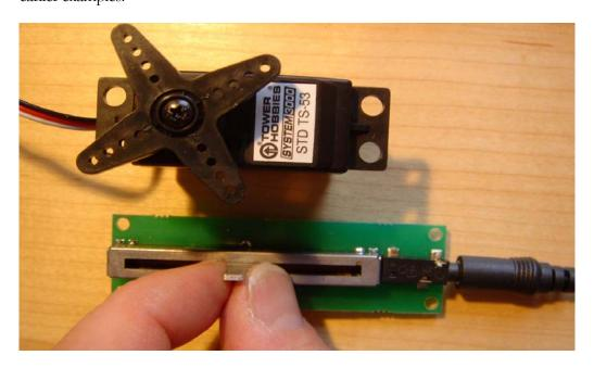
As before, plug a sensor such as a slider into Analog Input #1 of the Phidget InterfaceKit. Using the USB cable, plug the Phidget InterfaceKit into a USB port on your computer. Using another USB cable, plug the Phidget Servo into another USB port on your computer.
