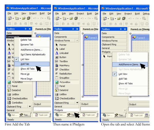
Using the Customize Toolbox, add the Grouplab.Phidget.dll. Click the Browse button (bottom right of the window on the following figure), and navigate to C:\Program Files\UofC\PhidgetSetup\. Select Grouplab.Phidgets.dll. All the phidgets components will now appear within your Customize Toolbox window, as shown below.
