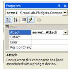
**Insert the following code in the servol\_Attach event handler.** The Attach event is raised when the servo device is seen by the system (i.e., when you start the program if the servo is plugged in, or if you plug in the servo after the program has been started. Through the code below, the servol\_Attach event handler will just rotate the 1<sup>st</sup> servo motor (counting from 0) to a random position between 0 and 180 degrees by setting that motor's Position property.
