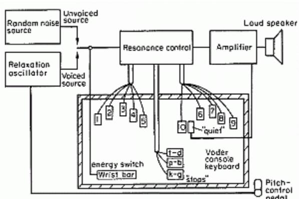
**Figure 3** A block schematic of Homer Dudley's VODER [2].
