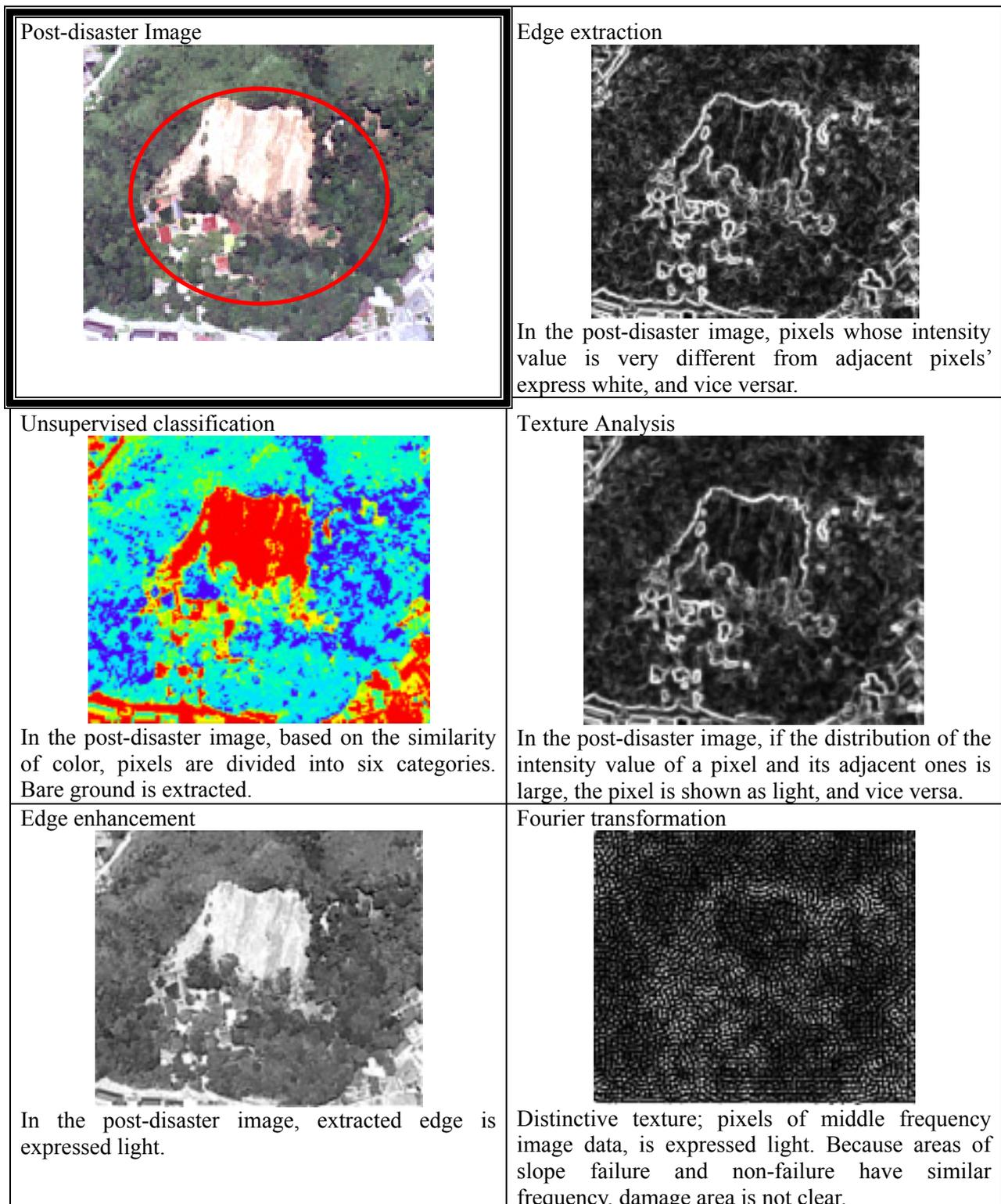
Fig.5 Result to apply image processing to areal-type damage
