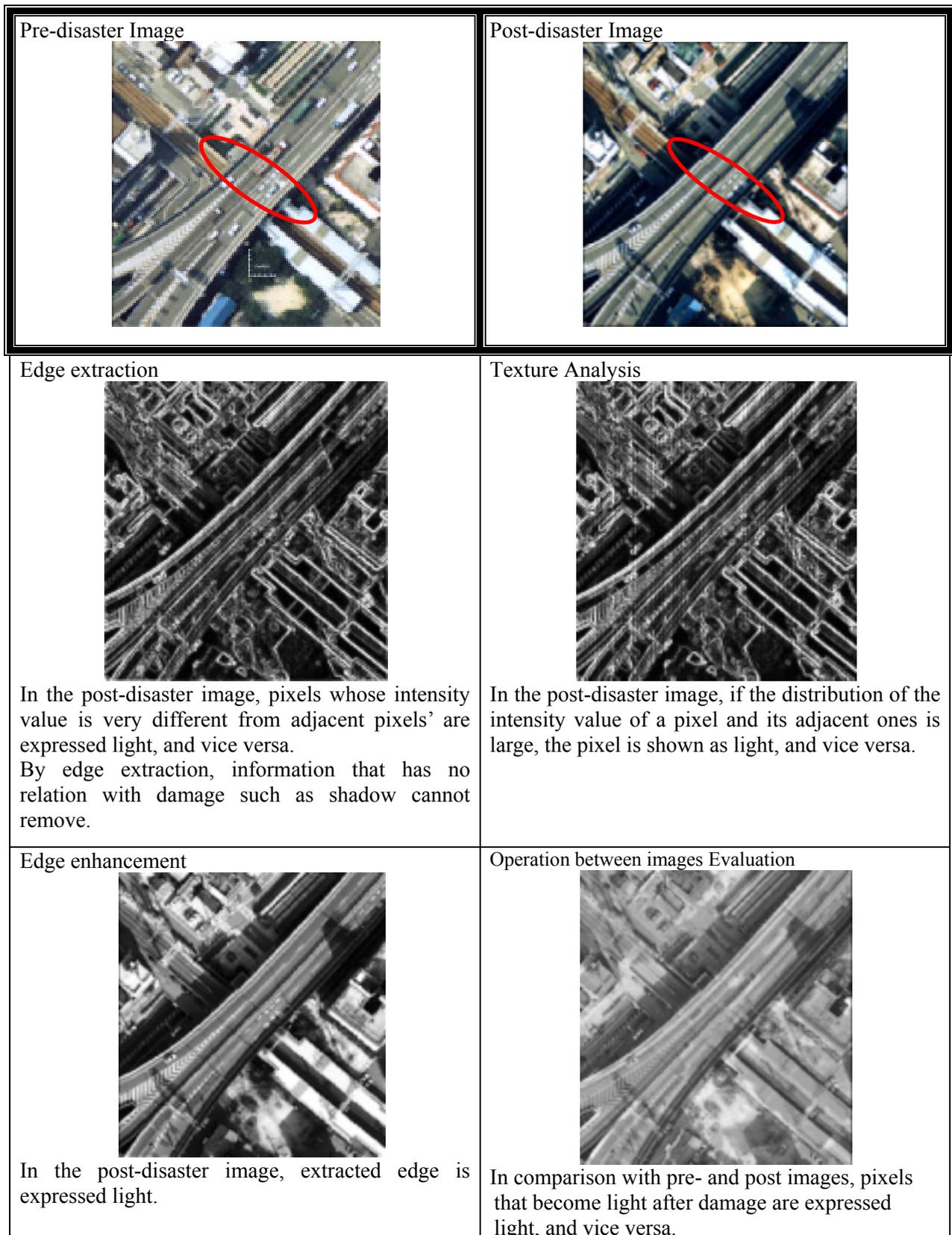
Fig.4 Result to apply image processing to liner-type damage
