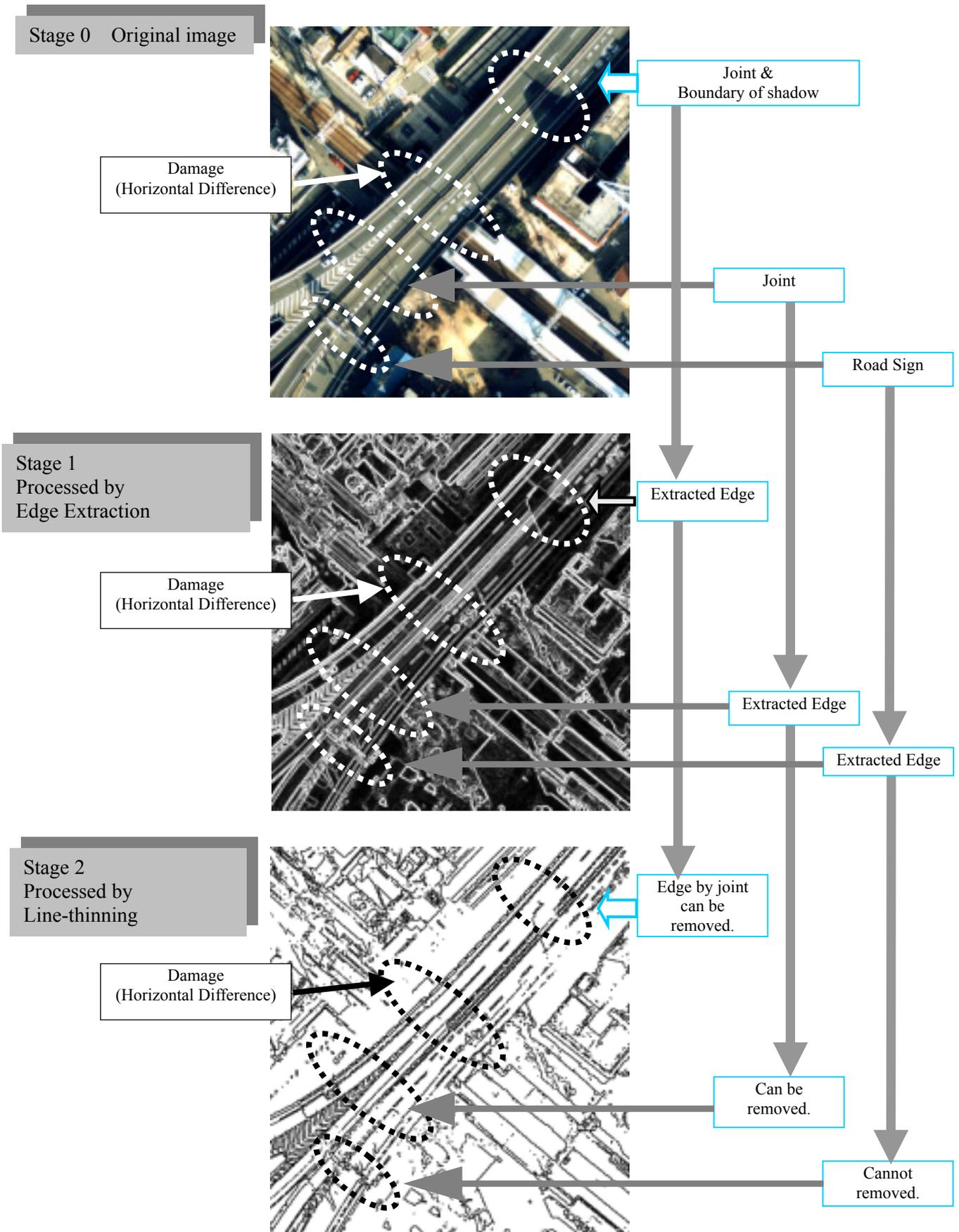
Fig.3 Combination of image processing to improve visibility of damage
