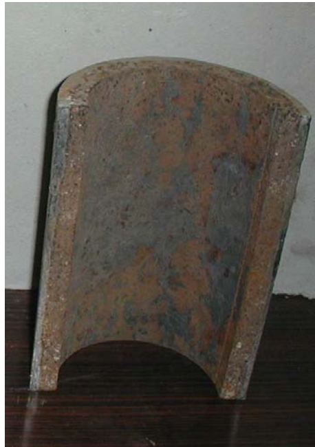
Bimetallic Pipe (Outer layer – Stainless steel, Inner layer – mild steel)
