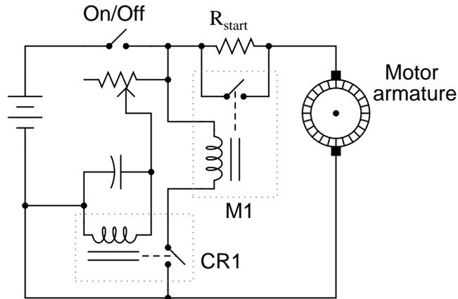
The relay labeled "M1" is a large "contactor" designed to shunt the motor's current around the start-up resistor. It requires at least a few amps of current through its coil to energize.
