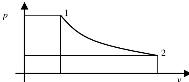
$w$  is the area under the process path.  $p_1v_1$  is the area of the rectangle between the origin and state 1.  $p_2v_2$  is the area of the rectangle between the origin and state 2, and  $w_s$  is the area to the left of the process path.
