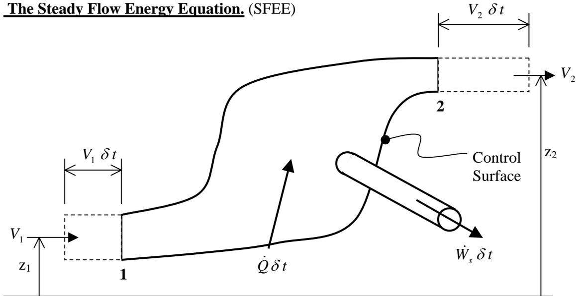
The sketch above shows a piece of equipment such as a boiler, engine, pump, etc. through which fluid steadily flows. The fluid enters the equipment with velocity  $V_1$  at an inlet **1** with area  $A_1$  and leaves with velocity  $V_2$  by an exhaust at **2** with area  $A_2$ . The heights of the inlet and exhaust above some reference datum are  $z_1$  and  $z_2$  respectively.
