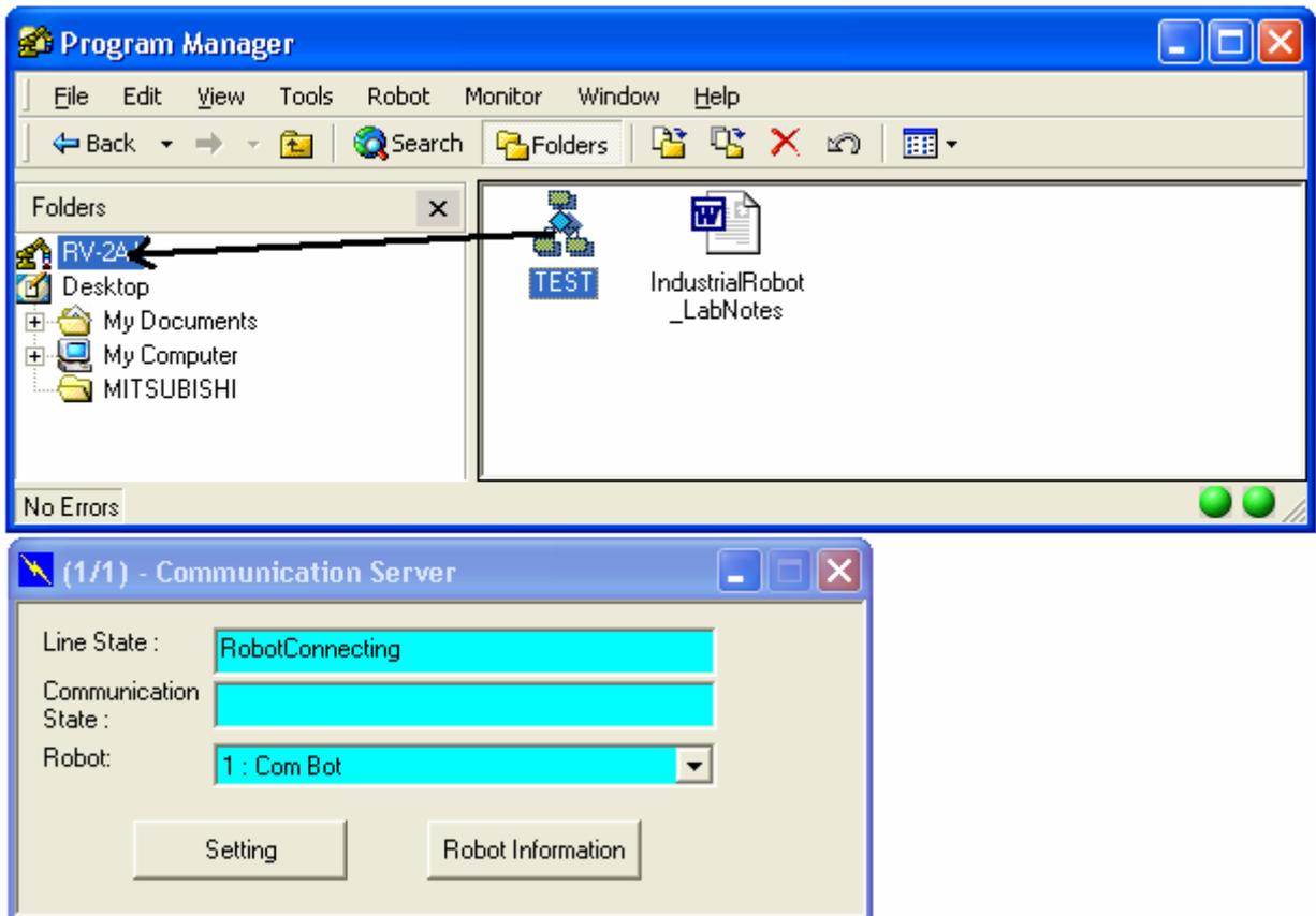
Figure 3 – Running a MELFA Basic programme from the PC
