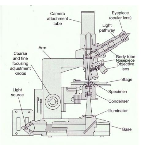
Figure: 2.1 Schematic diagram of a compound light microscope. The arrow indicates the path of light through the microscope
